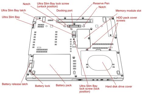
Figure 2-5 The underside of the computer
